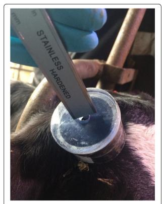
**Fig. 1** Methodology used to measure horn bud height showing the depth gauge of the calliper (model 49–923-150; Linear Tools, UK) positioned through the aperture of the cylinder (diameter 43 mm; height 30.85 mm) when placed over the horn bud
